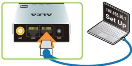
Then Open your web browser, and type-in "[alfa.myalfasetup.com](http://alfa.myalfasetup.com)" or "**192.168.36.1**" in the address bar.
